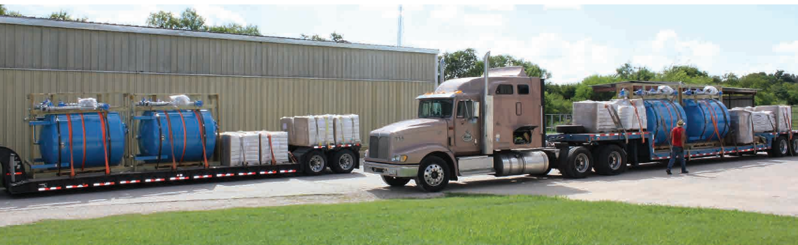
Quad 72"x72" Progressive Flow Water Softeners with Watts diaphragm valves.
